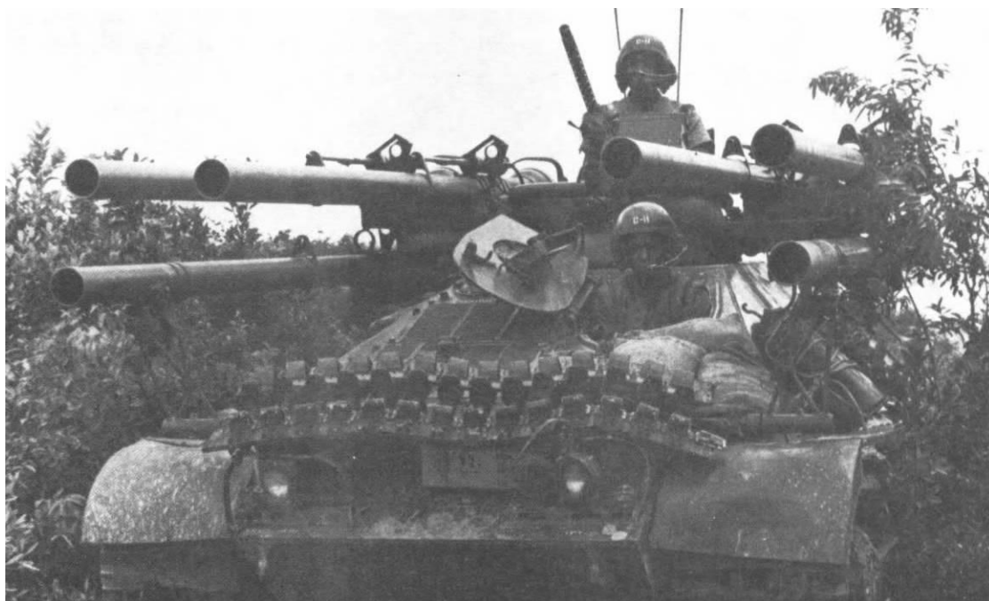
Two Ontos platoons of the 3d Antitank Battalion were on hand at Khe Sanh. The Ontos sports six 106mm recoilless rifles with coaxially mounted .50 caliber spotting rifles. (USMC Photo A369169)
