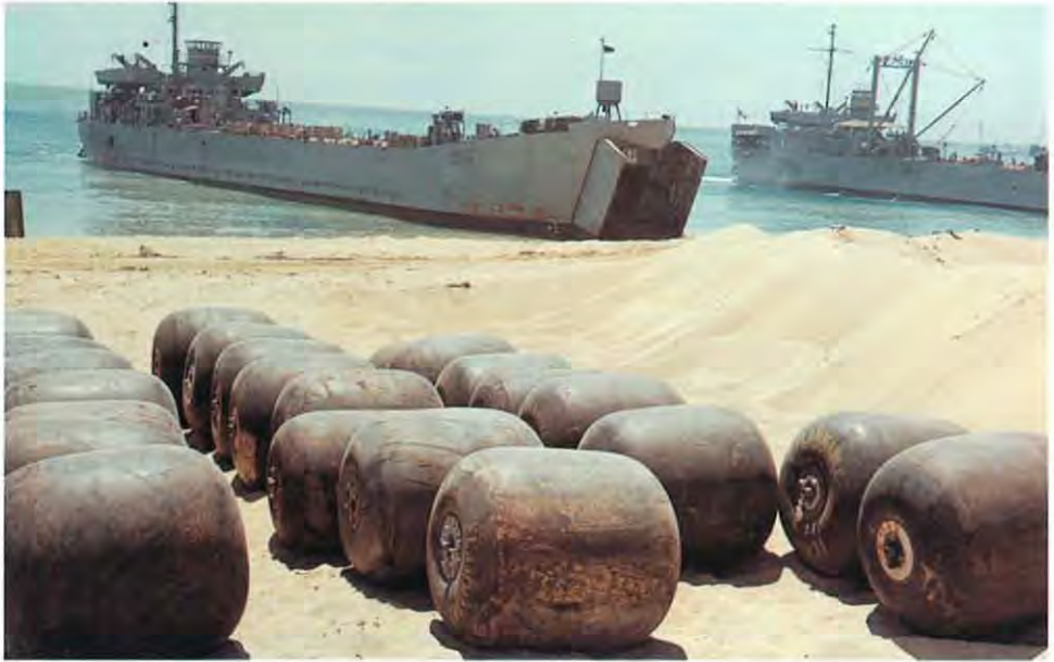
LSTs at RAZORBACK Beach. In the foreground, 500-gallon rubber fuel bladders are lined up on the sand.
